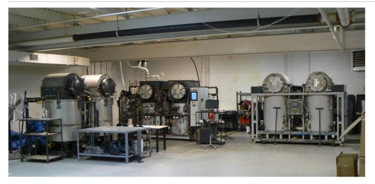
ly. In addition, there is the Electrochemical Oxidation (EO) unit for highly concentrated wastewater or for the removal of dissolved organics; the Oxidant Decomposition (OD) unit to reduce any residual oxidant content; the Bead Filter (BF) unit to remove all traces of residual turbidity; and several separators for the removal of large suspended solids, free oil, and/or residual organics.
