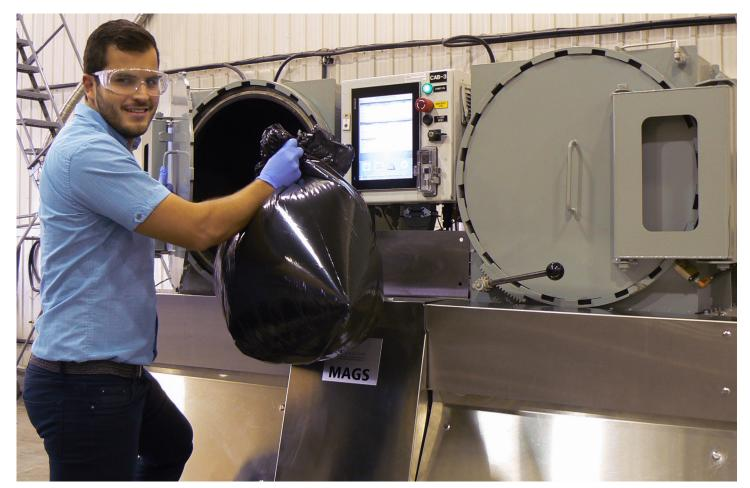
organic materials into thermal energy for use by the site where the materials are generated. Waste streams that can easily be converted into energy by MAGS, without the need for segregation, include, but are not limited to, paper/cardboard, plastics, food, oily rags, oils, and sludges.
