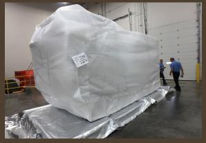
*Piece number one of a five-piece pharmaceutical manufacturing line for shipment overseas, ready to be vapor barrier protected*
