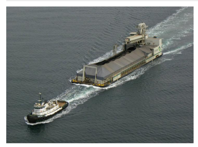
of three 320'-long steel bridge sections, each weighing about 700 tons, along with two 100-ton beams to New Jersey. The components are part of the new Wittpenn Bridge across New Jersey's Hackensack River. They were manufactured by Vigor Works, loaded onto Foss's barge, The American Trader on the Columbia River, then towed by the Lauren Foss south down the coast, and through the Panama Canal before heading back north to the U.S. East Coast.
